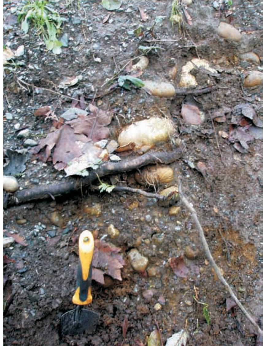
Photo 2. Silty sand and gravel on Stoney Creek channel bank.
