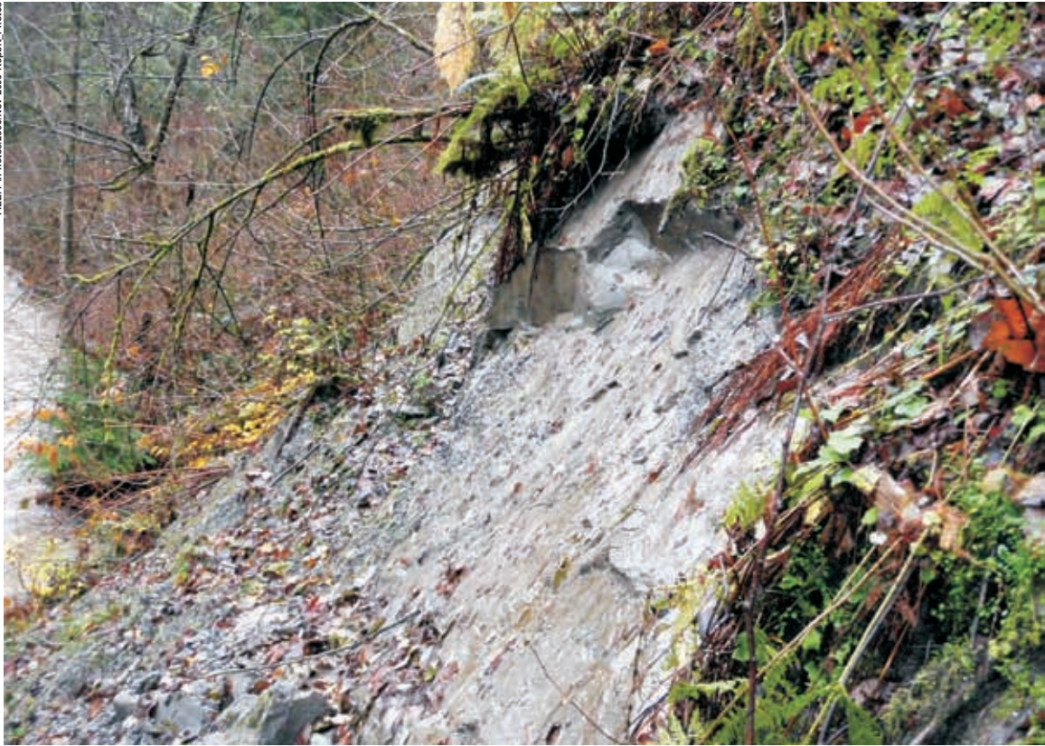
Photo 11. Clayburn Creek eroding toe of slope. Note blocks of fine-grained till or glaciomarine silt and clay spalling off scarp.
