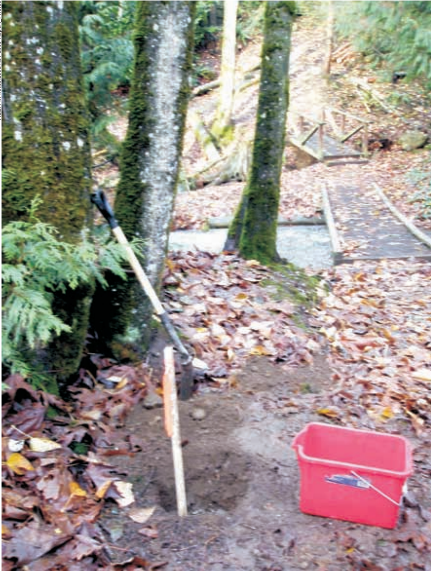
Photo 9. Percolation test set-up at McKee trial (Location 3).
