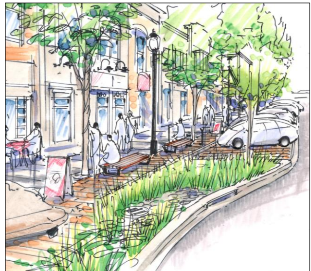
Figure 77 – Bioswale Stormwater Infrastructure
